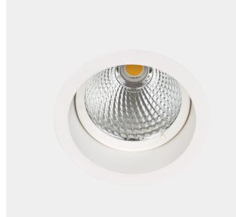
Our Trimo range of downlights guarantees a minimum of stray light. This is accomplished by using a recessed LED light source. This model requires a hole dimension of 112mm in diameter making it very versatile providing very powerful light. The Trimo Mini has a 18i3 connector and is supplied with a variety of connector solutions.
