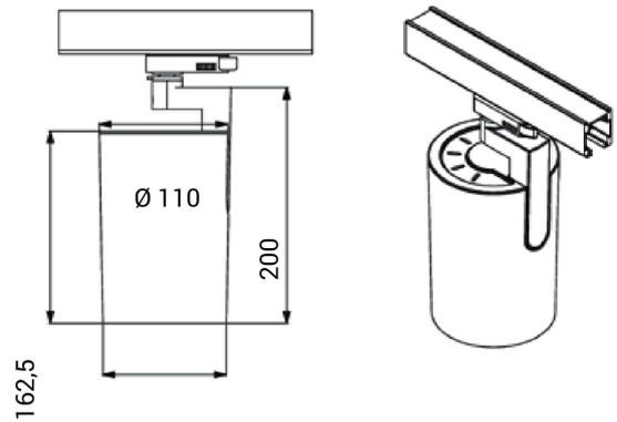
Ray Mini uses the possibilities created by new technology. The LED driver is mounted inside the luminaire body. This gives us a slim design combined with a powerful lightoutput that can be easily adjusted in all directions to meet all needs. Ray Mini can be tilted 90 degrees and rotated 350 degrees its own axis. To create further opportunities to play with light you can mount a diffuser on the luminaire, this can be ordered separately.
