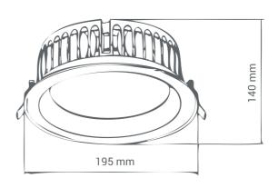
This series of IP44 downlights is named Auriga. Thanks to the IP44 rating the luminaire is very well suitable to outdoor use. Auriga is supplied with 2m cable for power connection.
