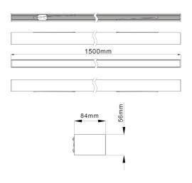
LEDline is a modern linear LED system for seamless lighting. It is based on modular chassis details allowing for seamless extensions through both straight connectors, 90 degrees corners and X-crosses. This allows light designers to make tailor fit lighting systems in an easy manner. The chassis details assure easy installation without failures. Add 1 pc 8050-05 for each mains supply (each row or standalone). Also add mounting accessories.
