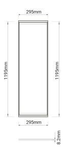
Panel LED is a light fixture for interior use. It is constructed for fitting in to suspended ceilings. Panel LEDs can be installed as a pendant or mounted on ceiling surfaces. The Panel LED has an opal or micro prismatic diffusor.
