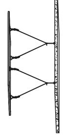
3. Fasten the Y rope end with the easy snap hooks. Use 3 pcs Y rope if 1195mm length.
