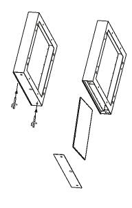
2. Snap the light in the ceiling bracket, then fasten the side panel with screws.
