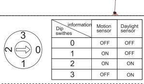
Adjust the dip switch to the module by screwdriver.
