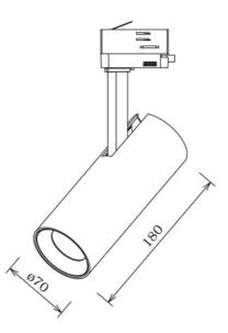
The Cylinder uses the possibilities created by new technology. The LED driver is mounted inside the luminare body. This gives us a slim design combined with a powerful light output that can be easily adjusted in all directions to meet all needs. Cylinder can be tilted 90 degrees and rotated 350 degrees its own axis. To create further opportunities to "play" with light you can mount a diffuser on the luminaire, this can be ordered separately.
