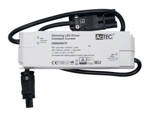
Phasecut driver for Panel Max 45W 900mA 22-40V Primary side18i3 male connector Secondary side EPN0034 connector
