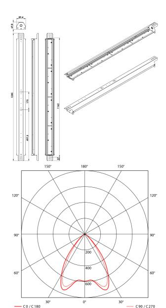
Bladeline Z is a highly efficient LED luminare with up to 179lm/w. Due to fact that it may be installed surface mounted on the ceiling or on electrical tracks makes it highly flexible. Can be opened without using tools and it has the electric connectors on quick fit clamps. The Bladeline Z is made from galvanized steel with medium or wide beam (75° and 90°) optic in 42W or 75W versions.
