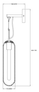
Tubus wall mounted luminaire with opal glass. Delivered with black canopy and leather strap.
