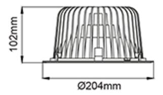
Leila C is a highly efficient downlight with 126 lm/w. With wide beam angle and rotationally symmetric light distribution, it`s suitable for all place that requires high lumen output. Can be delivered with on / off, phasecut or DALI2 driver. See accessories for suitable driver.
