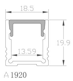
Black Aluminum profile for surface mounting. Includes opal cover, 2pcs end cap, 2pcs end cap with hole for cable and mounting clips.
