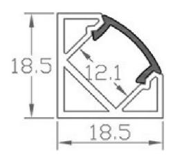
Corner profile in aluminium that can be used both for directly and indirectly lighting. Fits most of our LED-strips. Opal cover, mounting clips, screws and end caps are included.
