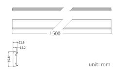
Blank cover to use on Trunk track. If trunk luminaire is used next to blank cover, use Trunk Cover - CFA-BC00-3 to avoid stray light.
