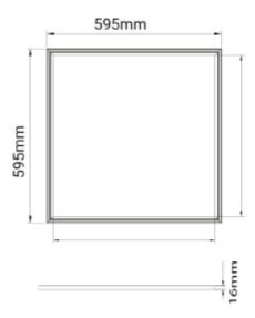
Panel with RGB. Need 24V driver and RGB controller. White wire is common +, red wire is Red, green wire is Green and black wire is Blue.
