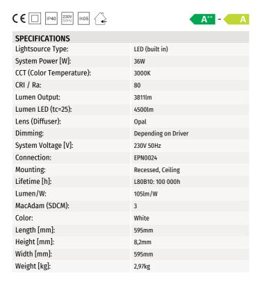
Panel LED is a light fixture for interior use. It is constructed for fitting in to suspended ceilings. Panel LEDs can be installed as a pendant or mounted on ceiling surfaces. The Panel LED has an opal or micro prismatic diffusor. Choose between ON/OFF, Phase-Cut or DALI2 (CLO, Corridor, Push dim and Ready2mains) driver. See accessories for detailed information.
