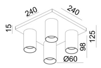
Tania Mini S4 is a small quadruple spotlight modern and contemporary design for surface mounting. GU10 light source not included. Gold front ring can be purchased separately.
