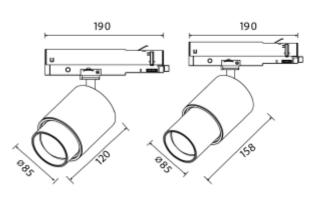
The unique zoom patent makes it possible to vary the beam angel between 6 and 60 degrees making this model highly versatile. The Zoom is available in both black and white versions and is made from robust die-cast aluminum.
