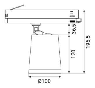
Cone shaped spotlight with high lumen efficiency for use in 3-circuit track. Available in black and white color with 3000K and CRI 90.
