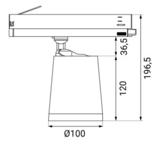
Cone shaped spotlight with high lumen efficiency for use in 3-circuit track. With honeycom filter.
