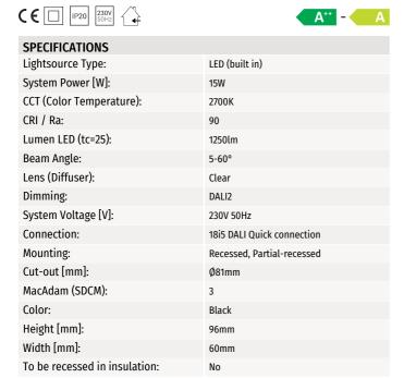
Zoom Recessed, is relatively small downlight with a cut-out size of Ø81mm. The unique zoom patent makes it possible to vary the beam angel between 5 - and 60 degrees making this model highly versatile. The Zoom Recessed is available in both 2700 and 3000 Kelvin and is made from robust die-cast aluminum. Tiltable 25° Please see the table for technical details.
