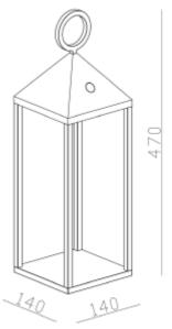
Beautiful outdoor lamp for long summer nights! The fixture is produced in die-cast aluminium and powder coated to last outdoors. 9 hours work time and 5-7 charge time operated by 2 x 220mAh lithium battery. Dimmable by touch switch to create the atmosphere you like.
