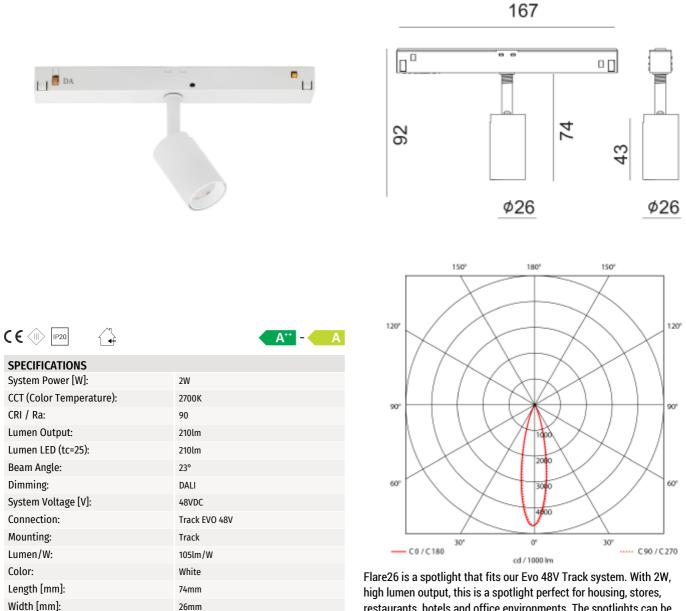
high lumen output, this is a spotlight perfect for housing, stores, restaurants, hotels and office environments. The spotlights can be adjusted in all angles to fit every need. Can be tilted 90 degrees and 350 degrees rotatable around its own axis.
