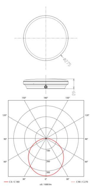
Dimmable surface mounted ceiling light with PC diffuser and even light output. IP54 waterproof structural design, its an ideal replacement for wet locations. Comes with a switch option between 2700K(default)and 3000K. Dimmable by phasecut or DALI2. QuickConnect for easy installation.
