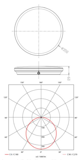
Surface mounted ceiling light with emergencylight, microwave sensor and CCT switch (2700K-3000K). 3h emergencylight and selftest. Factory setting Detection Area: 100% holdt Time: 5S Daylight Sensor: Disable Standby dim level: 0% Stand.by period: - See installation manual for alternative sensor settings.
