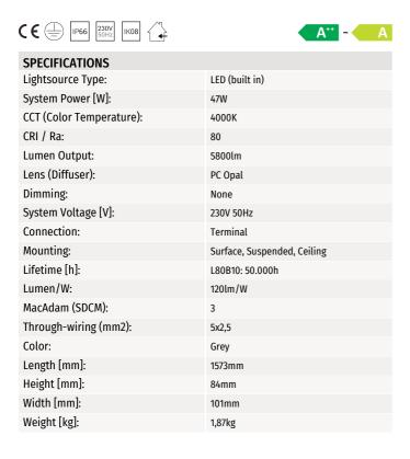
Duna is a sealed industrial light fixture for ceiling surface mounting, indoor or outdoor under a roof. Duna is classified in accordance with IP66 / IK08. The light fixture is made from robust fiberglass and is equipped with a semi-opal PC diffuser. Can be used together with 10184745 as slave luminaire (5pcs can be connected to one master).
