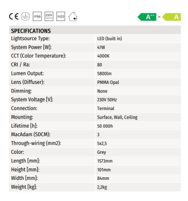
Duna is a sealed industrial light fixture for ceiling surface mounting, indoor or outdoor under a roof. Duna is classified in accordance with IP66 / IK03. The light fixture is made from robust fiberglass and is equipped with a PMMA diffuser. 5x2,5mm2 PG through-wiring. Suitable for use in carwash.
