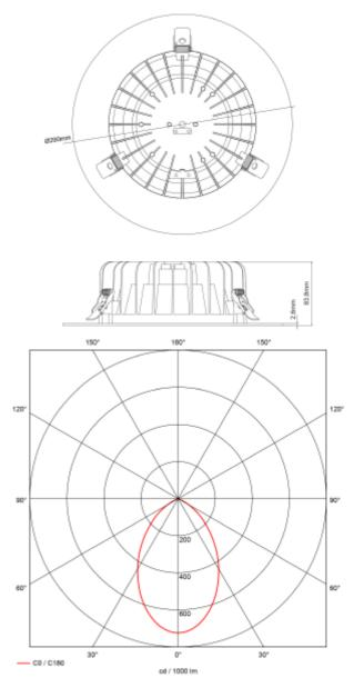
Leila R with cut out Ø240-270mm. Developed to change from halogen to downlight with latest LED technology. High Efficiency, easy installation. Delivered without driver. See accessories for correct driver-
