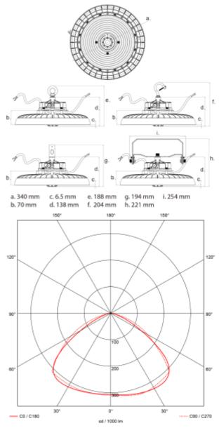
UFO U High Bay is a robust and versatile luminaire with high performance. With IP65 and IK08 classification, it can be used in most conditions. Comes with 1-10V dimming. PIR or Microwave sensor can be easily retrofitted. This product is also available with a PIR sensor featuring wireless communication between luminaires, using the Norlux Wireless Connect system for control. See accessories for sensor module.
