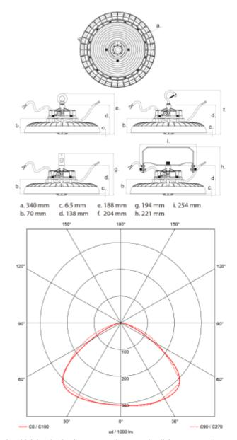
Ufo U high bay is absolute top-notch concerning light output and mechanical strength. The luminaire is classified accordance to the IP65 norm. This makes UFO B very suitable for use in tough conditions. The light output from the UFO B is >160 lm/W, makes this a perfect choice. Add a PIR or microwave sensor to make your light control more cost efficient. Ufo B high Bay are delivered with 1-10W / PWM dimming. Change effect by dip-switch 200W = 35900lm 150W = 26000lm 120W = 21400lm
