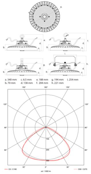
Ufo U high bay is absolute top-notch concerning light output and mechanical strength. The luminaire is classified accordance to the IP65 norm. This makes UFO B very suitable for use in tough conditions. The light output from the UFO B is >160 lm/W, makes this a perfect choice. Add a PIR or microwave sensor to make your light control more cost efficient. Ufo B high Bay are delivered with 1-10W / PWM dimming. Change effect by dip-switch 200W = 35900lm 150W = 26000lm 120W = 21400lm
