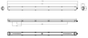
Stream Y is a sealed industrial light fixture for ceiling surface mounting or pendant installation. The Stream is classified in accordance with IP65 and 2,5mm2 through wire and is suited for use in garage, industry, and warehouse. The light fixture is equipped with a milky white (opal, polycarbonate) diffusor. Can be delivered with microwave sensor for wireless control between luminaires with Norlux Wireless Connect control.
