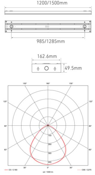
Uniplus is a surface mounted luminaire with the latest technology and opticts to ensure a high luminous efficiency and low glear. -Low glear UGR19 -Up to 150lm/w -Easy and fast installation. -Suspended installation (accessory) Efficiency can be adjusted by dip switch: 39W = 5670lm 34W = 5000lm (default setting) 28W = 4130lm 23W = 3470lm
