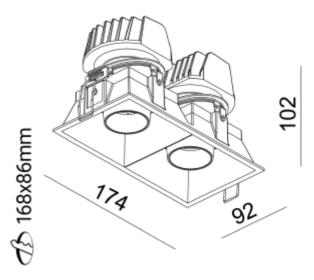
Make Double is a square downlight with Dim 2 Warm. The color temperature (K) can be adjusted between 1900K and 3000K. Rotatable 360° and tiltable 20°. Driver is not included and sold separately. See accessories for recommended drivers. Please note that the downlight comes with white front ring. Black front ring is sold separately.
