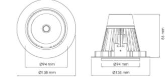
This is by far our most popular mini" downlight and it offers huge flexibility, tiltable up to 25 degrees. This downlight has a recessed light source giving a minimum of stray light. The Torres Mini can be supplied with a variety of connector solutions.
