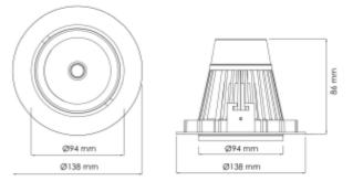
This is by far our most popular mini" downlight and it offers huge flexibility, tiltable up to 25 degrees. This downlight has a recessed light source giving a minimum of stray light. The Torres Mini can be supplied with a variety of connector solutions.
