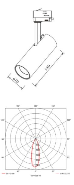
The Cylinder uses the possibilities created by new technology. The LED driver is mounted inside the luminare body. This gives us a slim design combined with a powerful light output that can be easily adjusted in all directions to meet all needs. Cylinder can be tilted 90 degrees and rotated 350 degrees its own axis. To create further opportunities to "play" with light you can mount a diffuser on the luminaire, this can be ordered separately.
