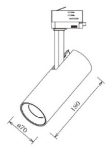
The Cylinder uses the possibilities created by new technology. The LED driver is mounted inside the luminare body. This gives us a slim design combined with a powerful light output that can be easily adjusted in all directions to meet all needs. Cylinder can be tilted 90 degrees and rotated 350 degrees its own axis. To create further opportunities to "play" with light you can mount a diffuser on the luminaire, this can be ordered separately.
