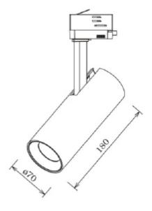
The Cylinder uses the possibilities created by new technology. The LED driver is mounted inside the luminare body. This gives us a slim design combined with a powerful light output that can be easily adjusted in all directions to meet all needs. Cylinder can be tilted 90 degrees and rotated 350 degrees its own axis. To create further opportunities to "play" with light you can mount a diffuser on the luminaire, this can be ordered separately.
