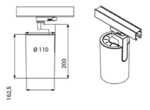
Ray Mini uses the possibillities created by new technology. The LED driver is mounted inside the luminare body. This gives us a slim design combined with a powerful lightoutput that can be easily adjusted in all directions to meet all needs. Ray Mini can be tilted 90 degrees and rotated 350 degrees its own axis. To create further opportunities to play with light you can mount a diffuser on the luminaire, this can be ordered separately.
