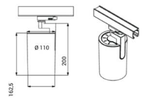
Ray Mini uses the possibilities created by new technology. The LED driver is mounted inside the luminare body. This gives us a slim design combined with a powerful lightoutput that can be easily adjusted in all directions to meet all needs. Ray Mini can be tilted 90 degrees and rotated 350 degrees its own axis. To create further opportunities to play with light you can mount a diffuser on the luminaire, this can be ordered separately.
