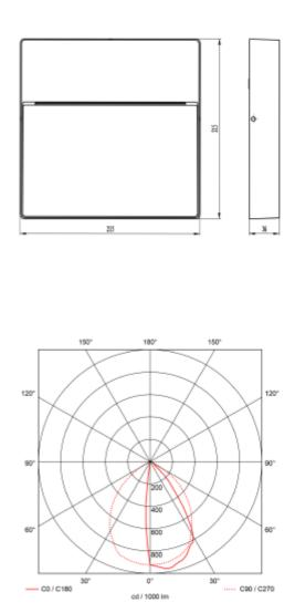
This luminaire has a robust construction and is made from die cast aluminum with a very durable anthracite grey surface. Chara Square is very suitable for use in exterior staircases and facades where you want discreet but good lighting.
