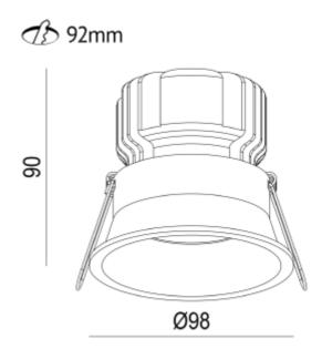
Ceto Fixed is a downlight with 15W effect and secluded light source. 36° beam angle and IP44 certified. Ceto Fixed is the natural choice if you are looking for an exclusive expression that provides a comfortable and good light. Dimmable phase-cut driver included.
