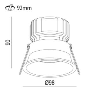
Ceto Fixed tunable white is a downlight with 15W effect and secluded light source. 36° beam angle and IP44 certified. CCT can be adjusted from 6000K to 2700K. Ceto Fixed is the natural choice if you are looking for an exclusive expression that provides a comfortable and good light. DALI DT8 driver included.
