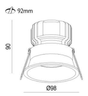
Ceto Fixed tunable white is a downlight with 15W effect and secluded light source. 36° beam angle and IP44 certified. CCT can be adjusted from6000K to 2700K. Ceto Fixed is the natural choice if you are looking for an exclusive expression that provides a comfortable and good light. DALI DT8 driver included.
