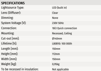
Seta Mini is a small and very flexible LED downlight offering great number of adjustment possibilities. The Seta Mini is supplied with a cable connector type 18i3- and can be delivered with a variety of connector options. The downlight is available in three different colors and with a wide range of reflectors. Rotatable 350° and tiltable 70°.
