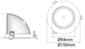
Seta Mini is a small and very flexible LED downlight offering great number of adjustment possibilities. The Seta Mini is supplied with a cable connector type 18i3- and can be delivered with a variety of connector options. The downlight is available in three different colors and with a wide range of reflectors. Rotatable 350° and tiltable 70°.
