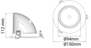
Seta Mini is a small and very flexible LED downlight offering great number of adjustment possibilities. The Seta Mini is supplied with a cable connector type 18i3- and can be delivered with a variety of connector options. The downlight is available in three different colors and with a wide range of reflectors. Rotatable 350° and tiltable 70°.
