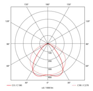
T-Line is our new luminaire for mounting directly into 3-phase track. By using DIP-switch on the wattage setting, you can adjust power to optimize your wattage setting. Choose between 35/40/45W. Preset is set at 50W. T-line comes in 3000K or 4000K with 90°, 120° or double asymmetric beam.
