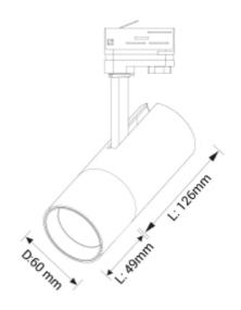
The Cylinder 60 has the LED driver included in the lamp head and is available for use in 1-circuit and 3-circuit tracks, both models are available with a Dim to Warm option. It can be tilted 90 degrees and rotated 350 degrees on its own axis and comes with a variety of accessories.
